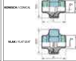
UNION CONICAL-FLAT SEAT BW / BW
